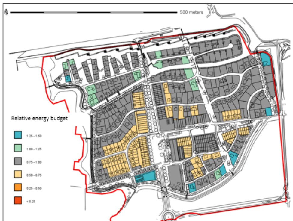
Figure 5. Optimal lot weights, where the weight and reference energy budget (-32 kWh/m/y) defines the maximum allowed heat extraction for each system.
